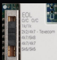
Built in EOL resistors
